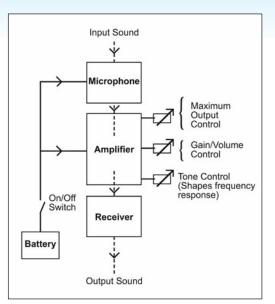
• There is a limit to the number of complex circuits at the signal processing stage and the more circuits there are the more chance of noise in the signal.
