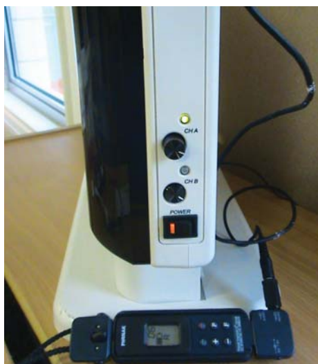
Redcat with Smartlink in re-broadcast mode. Note that the input to the Smartlink is to the microphone socket.
