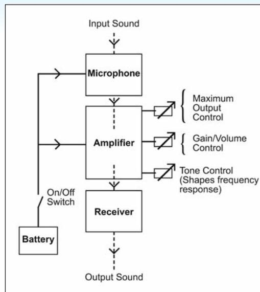
**Programmable hearing aids** use analogue signal processing but do have a digital chip that allows frequency response and output limiting to be altered by computer.
