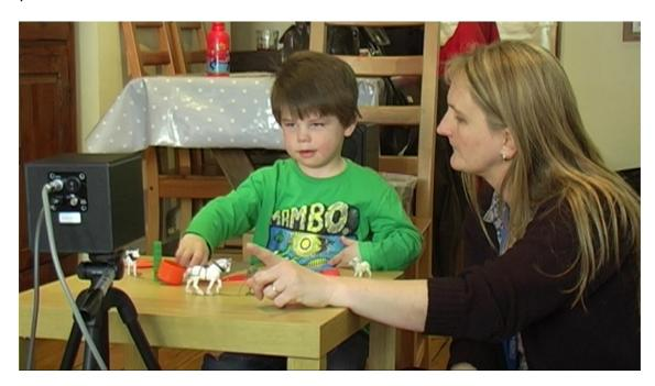
3. Seat the child at a distance of 75cm from, and facing, the loudspeaker (1), 0° azimuth, which will deliver the speech signals. Place the loudspeaker for delivering the noise signal directly behind the child, 180° azimuth, at a distance of 1m. Both loudspeakers should be at ear level.
