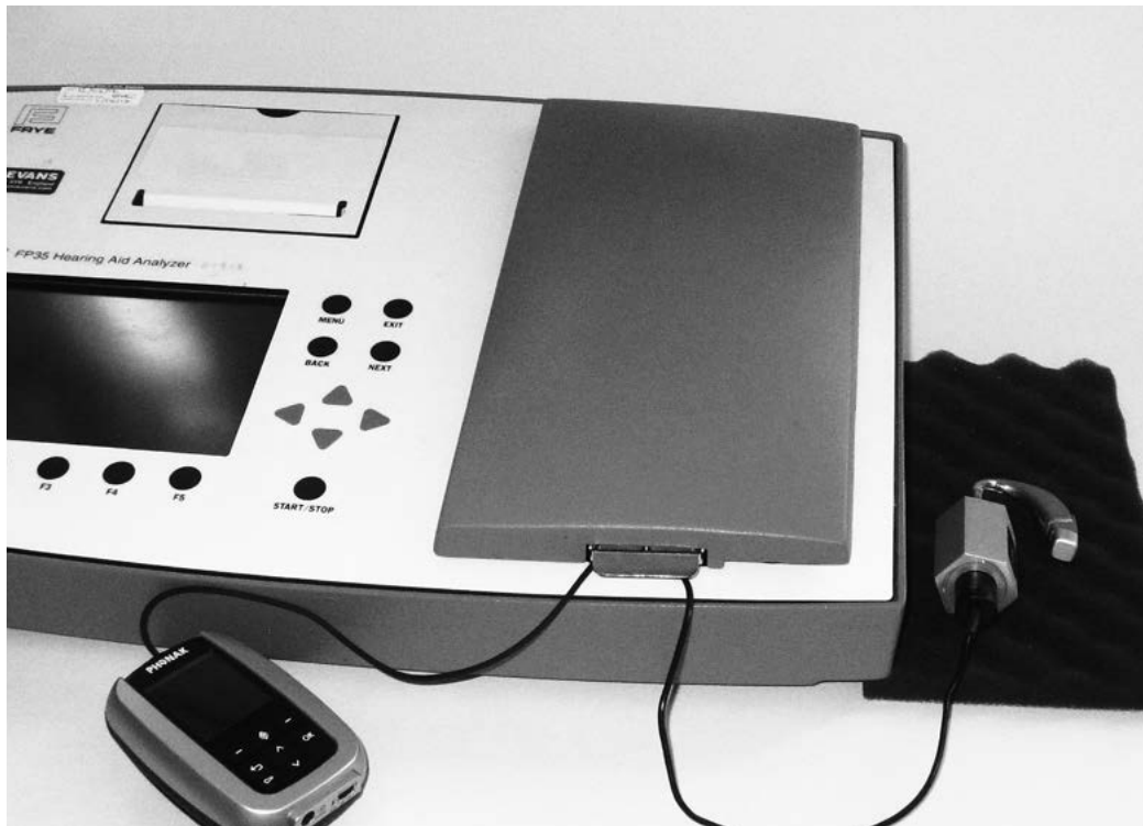
Test box in use for radio aid verification.
