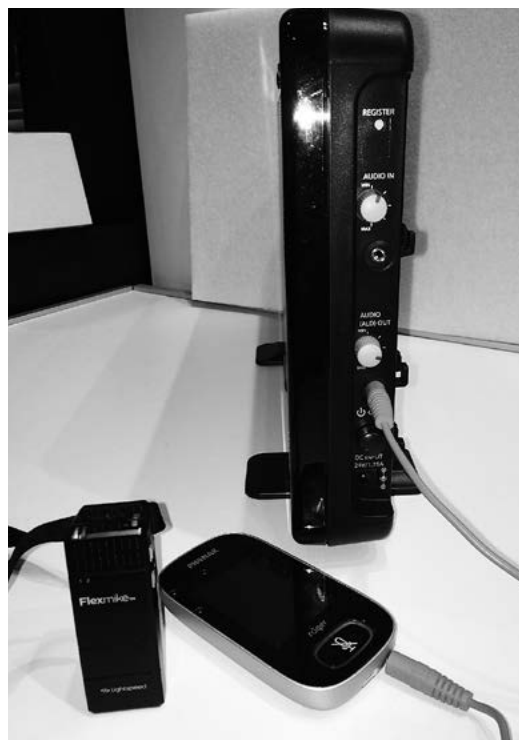
A personal radio aid transmitter connected to the soundfield system © PC Werth
