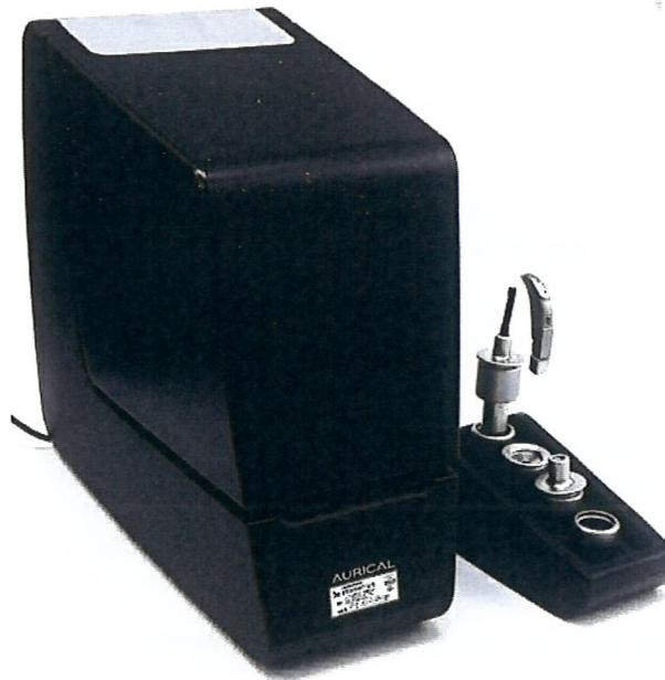
Test box in use for radio aid verification.
